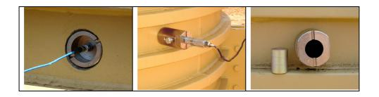
Figure 3 (from left to right) Reflected pressure sensor, overpressure sensor fixture and momentum gauge
