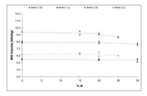
Figure 9 Mass Weighted Impulse
