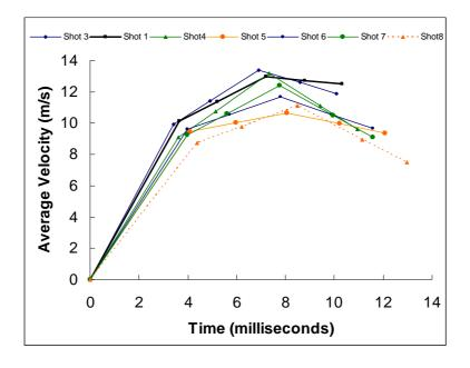
Figure 7 Momentum gauge average velocity measurements
